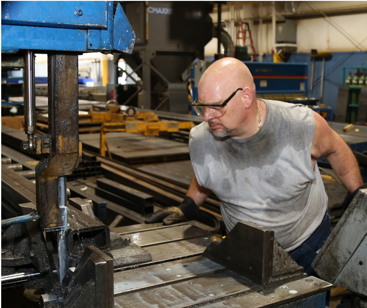
Kenneth Rogers, 52, of Mercer, a graduate of Butler County Community College’s manufacturing pre-apprenticeship program, observes a vertical semiautomatic band saw slicing 5-inch by 3-inch square structural steel tubing at Miller Industries, Hermitage, on Friday, June 1, 2018.
