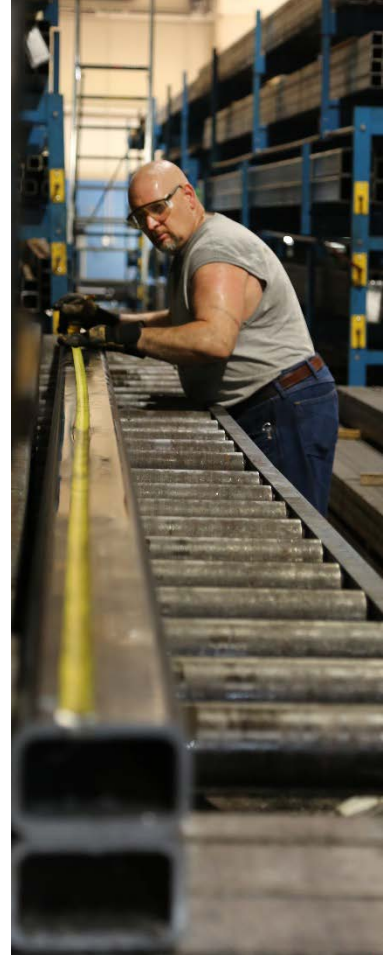
Kenneth Rogers, 52, of Mercer, a graduate of Butler County Community College's manufacturing pre-apprenticeship program, measures 5-inch by 3-inch square structural steel tubing at Miller Industries, Hermitage, on Friday, June 1, 2018.
